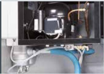
**Integrated filters and dryer**
