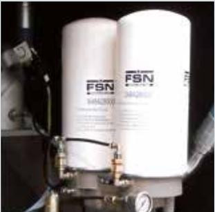
Storm 55 and 75 kW versions are equipped with double separator filter.
